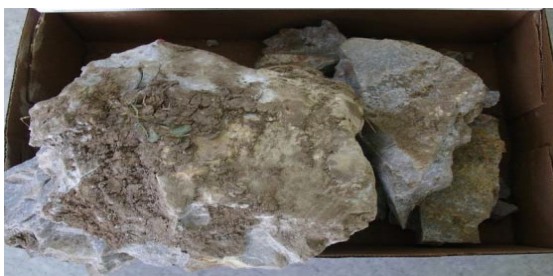
Example 1: Secondary school in the vicinity of a quarry with blocks landing in the playground approximately 300 m in front of the blast
