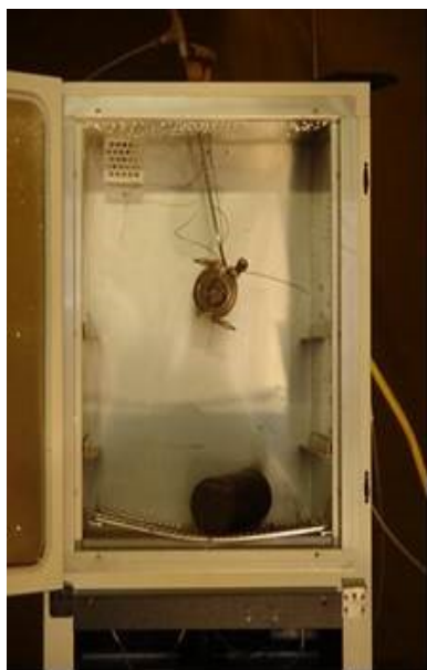
Figure 5 Damage to the Dewar apparatus after an experiment on unsensitised bulk ANWE Left: damage to the oven. Right: damaged (sheared neck) and undamaged Dewar vessels
