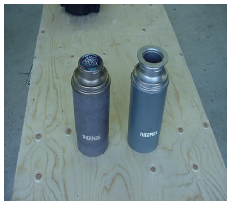
Figure 5 Damage to the Dewar apparatus after an experiment on unsensitised bulk ANWE Left: damage to the oven. Right: damaged (sheared neck) and undamaged Dewar vessels
