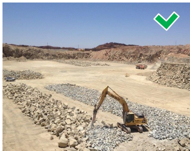
Figure 2: Recommended boulder hammering procedure.
