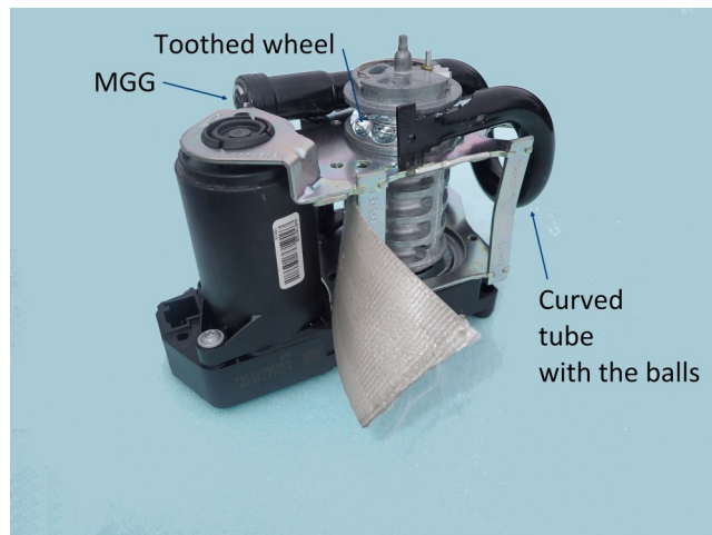
Photograph of the pretensioner mechanism with the MGG and the toothed wheel
