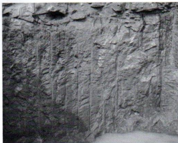
Figure 5 - Pre-split test Blast results in Creation of Fracture Plane
