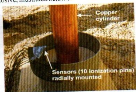
Figure 1 - Cylinder Expansion Test Set-up
