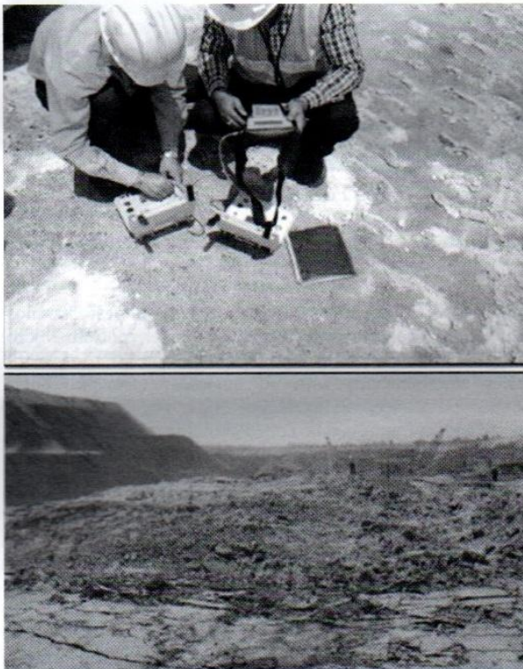
Figure 9 and 10 - Field checking of connectivity and blast result with Microdet-1 in a large coal mine
