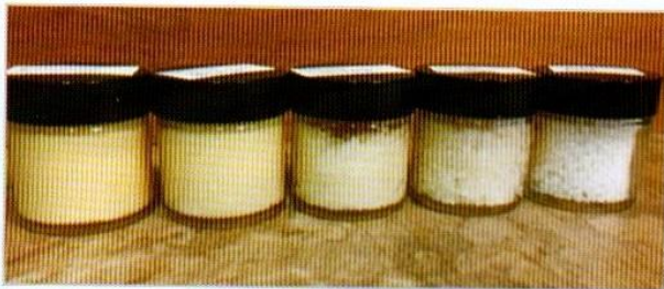
From left to right : Emulsion, Emulsion ANFO blends - 70/30 Blend, 50/50 Blend, 30/70 blend and ANFO.
