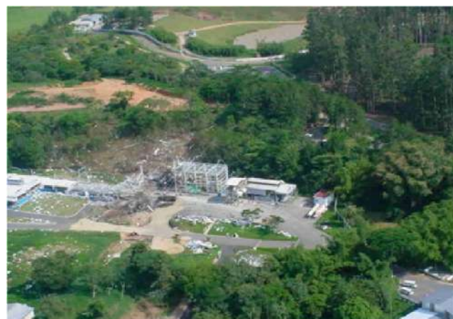
Fig.3 Explosion did not propagate beyond this point along the cartridge conveyor to the packing building. Which plant, which country?
