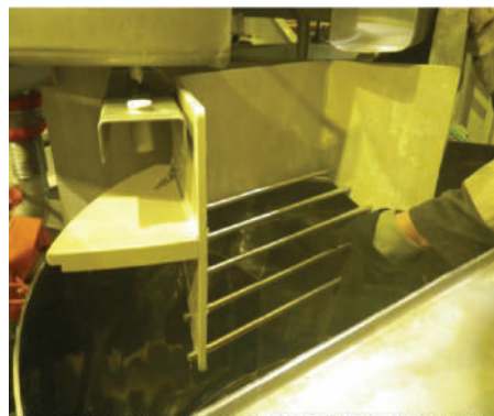
: Hopper/Breaker Bar Assembly in position without Slurry Vessel lid to hold it in place
