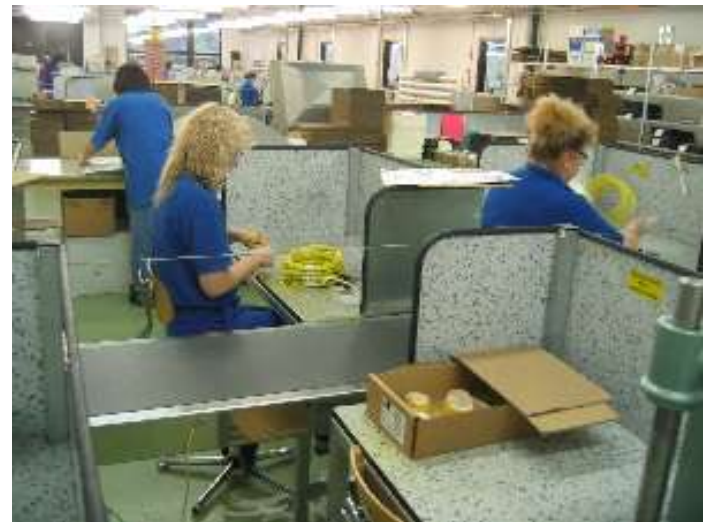
Fig. 4 Personnel handling explosives/initiating devices before the implementation of robotics and automation Which plant, which country
