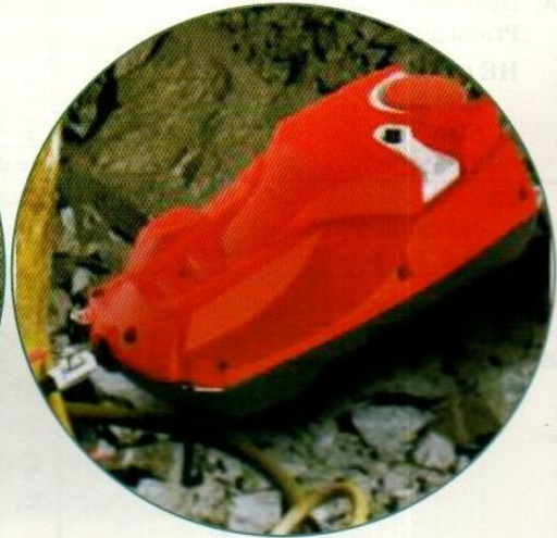
The pump is used in conjunction with bagged emulsion in the confined spaces found in Narrow Reef stopes and tunnels. The system effectively replaces packaged explosives.
