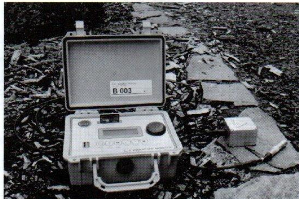
Figure 9 - Continuous Monitoring Blast Vibration meter with GPS included
