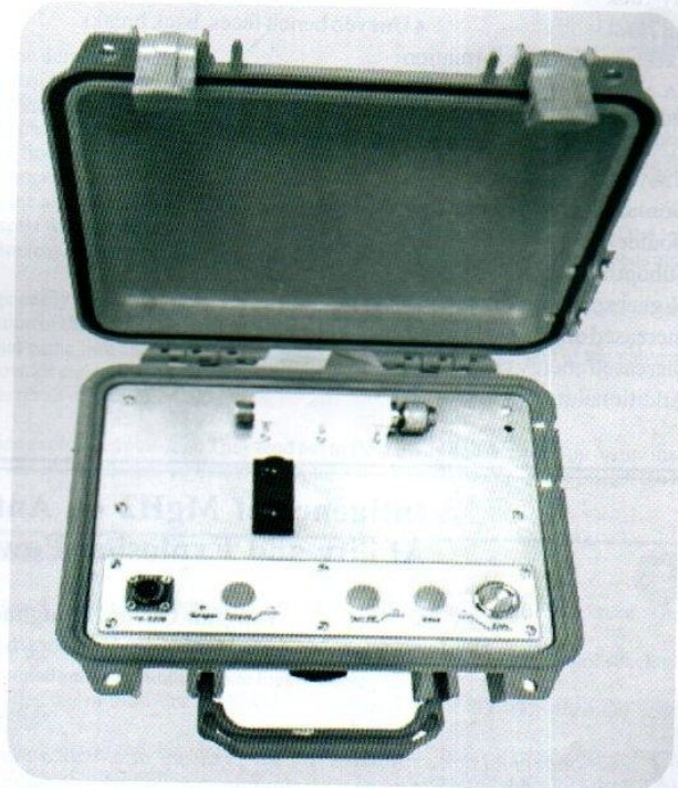
Figure - Actuating Unit - Retransmitter is designed for transmitting the data in the radio network in poor radio exchange conditions (remoteness, almost zero visibility, and presence of RFI - radio frequency interference)
