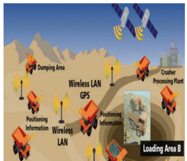
Figure 4: Working concept of FMS
