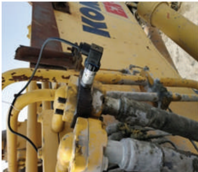
Figure 8 - Sensors fitted on hydraulic pressure lines
