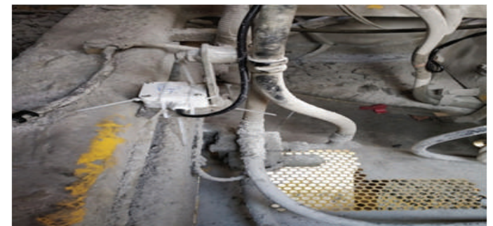
Figure 7 -Sensors fitted on Chassis of Excavator
