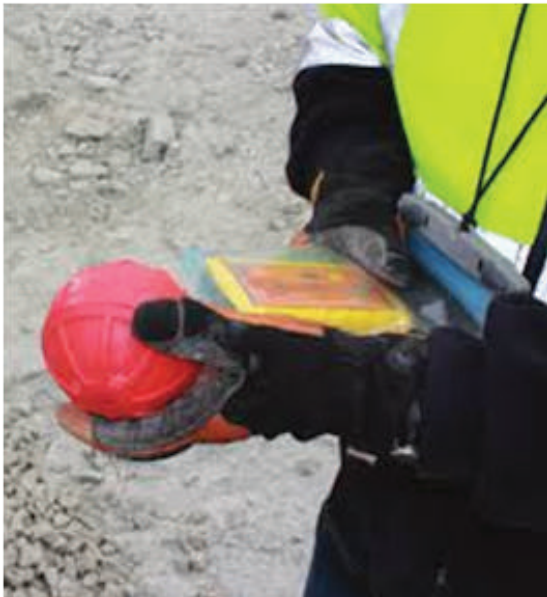
Figure-8: Blast Movement Monitor (image downloaded from google)
