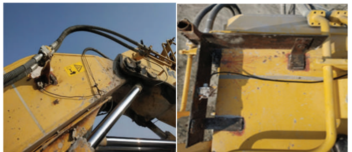
Figure 6:Sensors fitted on arm and boom of Excavator
