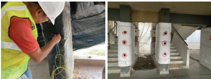
Figure 7: Loading of column at Alfa Serene and wrapping of the column of H 2 O Holy Faith Apartments
